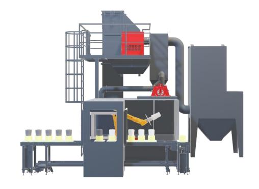
Example of automated workpiece loading on a hook
